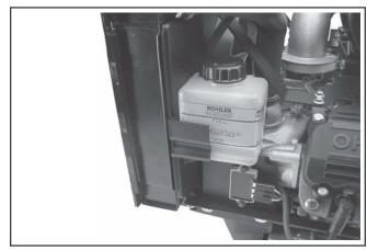
Figure 9. Overflow Reservoir Location.
